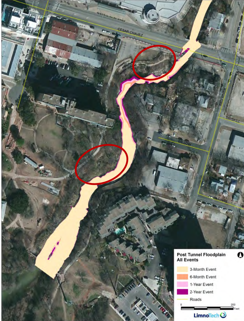
Post-Tunnel Wet Extents
